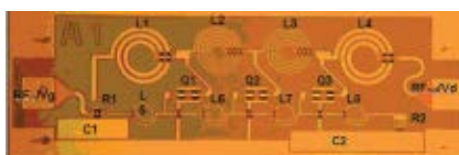
▲ Fig. 5 Microphotograph of the distributor amplifier chip.
