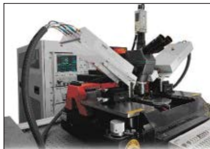
▲ Fig. 6 On-wafer measurements to 500 GHz with the ME7808C from Anritsu.
