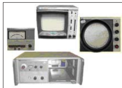
▲ Fig. 2 The HP8410 network analyzer mainframe and various plug-in modules.
