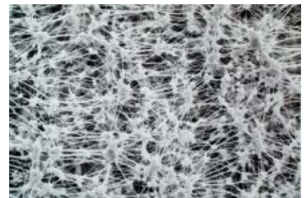
▲ Fig. 2 The "nodes and fibrils" of ePTFE.
