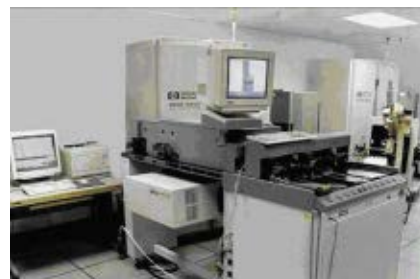
▲ Fig. 4 An early RFIC test station for high volume production.
