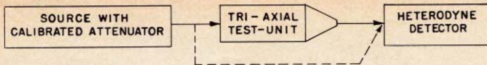
Figure 5—Block Diagram of the Measuring System.
